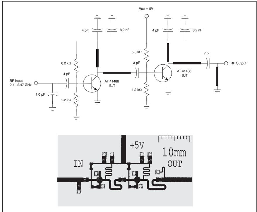
■ Figure 7. 2.4 GHz two-stage low noise amplifier (LNA) — circuit diagram (top) and board layout (bottom).
