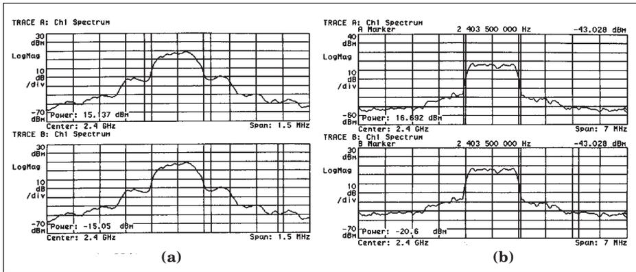
■ **Figure 20.** ACP measurement of the transceiver in transmit mode: (a) 384 kbps  $\pi/4$  DQPSK signal ( $-3$  dBm) with 380 kHz channel bandwidth; (b) 1.228 Mbps OQPSK spread spectrum signal ( $-3$  dBm) with 1.5 MHz channel bandwidth.
