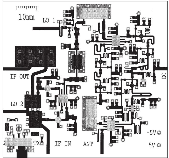
■ **Figure 15(a).** Circuit layout of the 2.4 GHz transceiver RF front-end.
