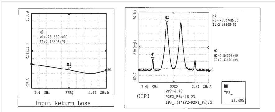
■ Figure 4. Measured input return loss and two-tone test of the 2.4 GHz two-stage power amplifier.
