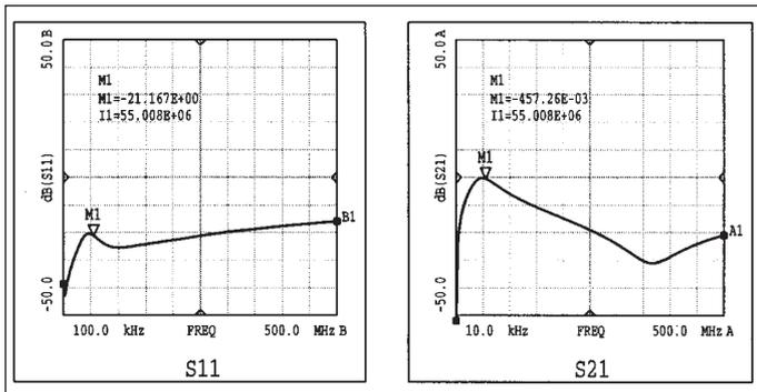
■ **Figure 14.** Measured characteristics of the 55 MHz 2nd IF bandpass filter (PIF-50).
