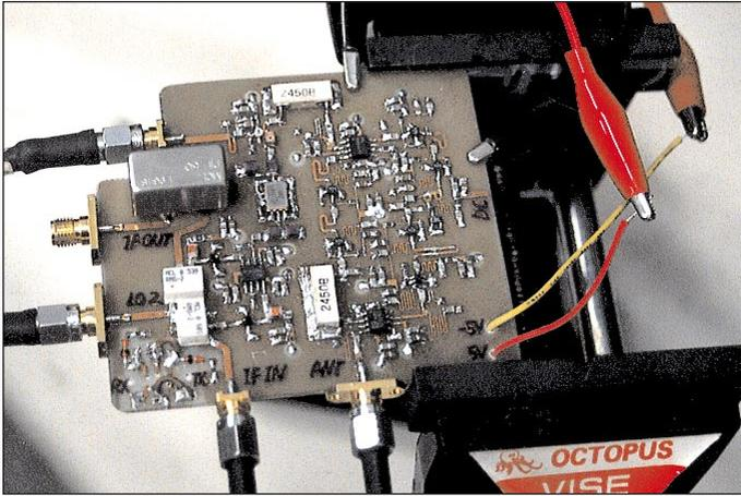
■ Figure 16(a). Photo showing connection of test cables to the RF transceiver board.
