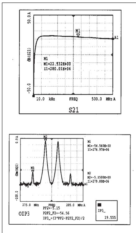
■ Figure 10. Measured characteristics of the 280 MHz 2nd IF amplifier (MAR-6).
