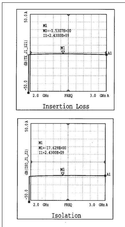
■ Figure 11. Measured characteristics of the T/R switch (MSTW-4-20).
