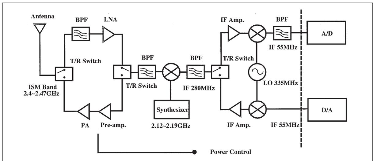
■ Figure 1. Block diagram of a 2.4 GHz transceiver front-end for digital wireless communications.
