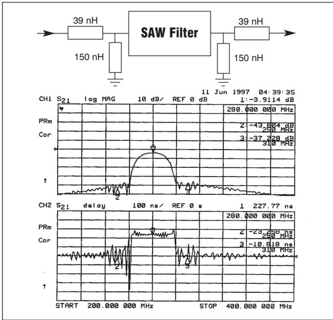
■ **Figure 13.** Measured characteristics of the 280 MHz band-pass filter (Toyocom SAW filter): Top is S21, bottom is group delay.
