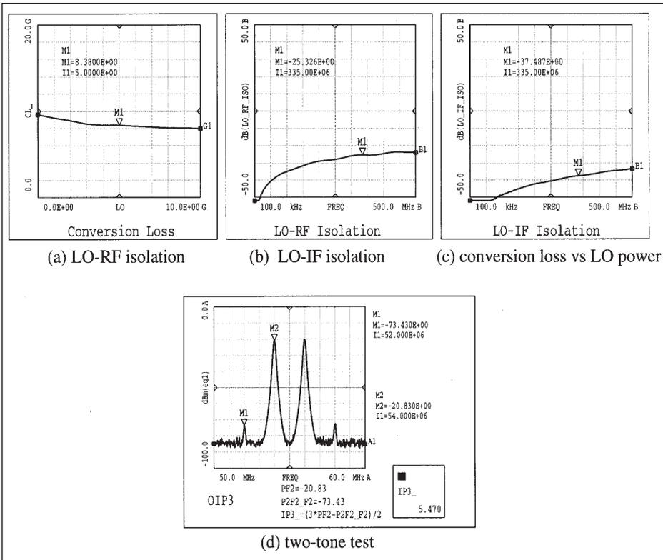
■ Figure 9. Measured characteristics of the 280 MHz 2nd IF mixer (Mini-Circuits RMS-2).
