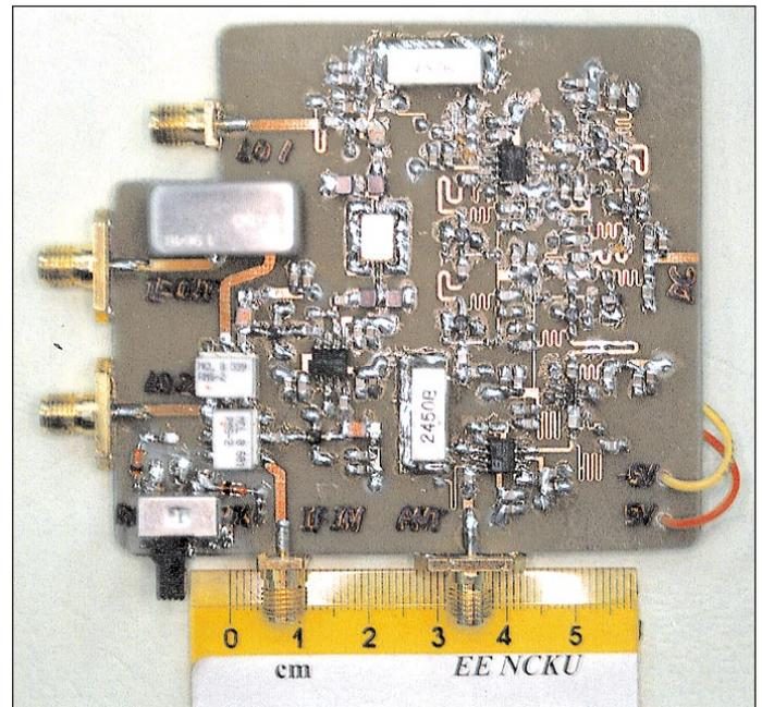
■ **Figure 15(b).** Photograph of the assembled transceiver (RF front-end, not including frequency synthesizer), as constructed on FR-4 board.
