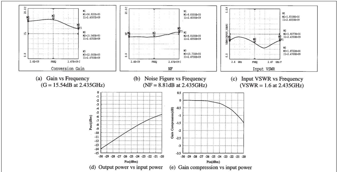
■ Figure 18. Measurement plots for the receive mode performance of the 2.4 GHz transceiver.
