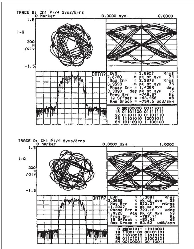
■ Figure 19. 384 kbps  $\pi/4$  DQPSK digital modulation measurement of the transceiver (top is transmit mode, bottom is receive mode).
