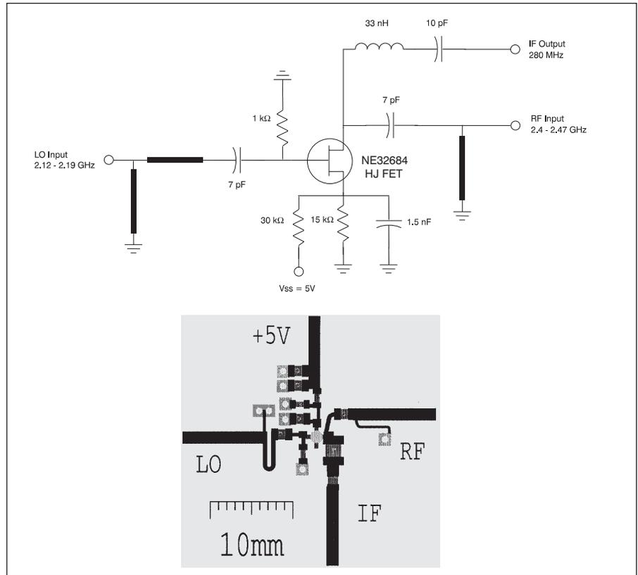
■ **Figure 5** 2.4 GHz single-ended resistive FET mixer — circuit diagram (top) and board layout (bottom).
