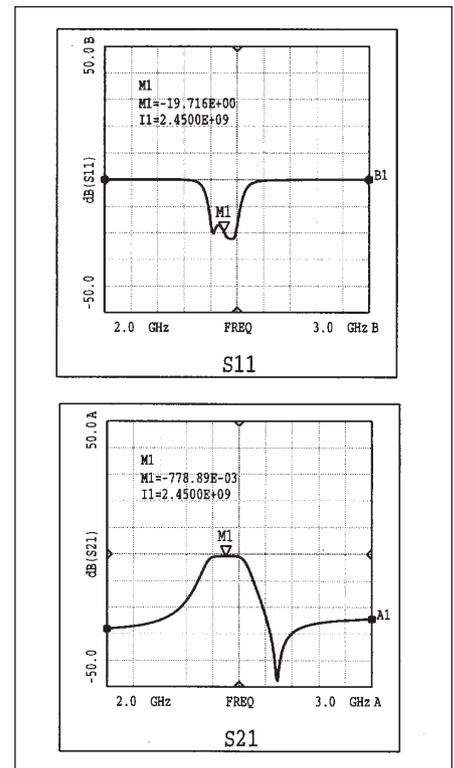
■ Figure 12. Measured characteristics of the 2.4 GHz bandpass filter (FDK 2450B).
