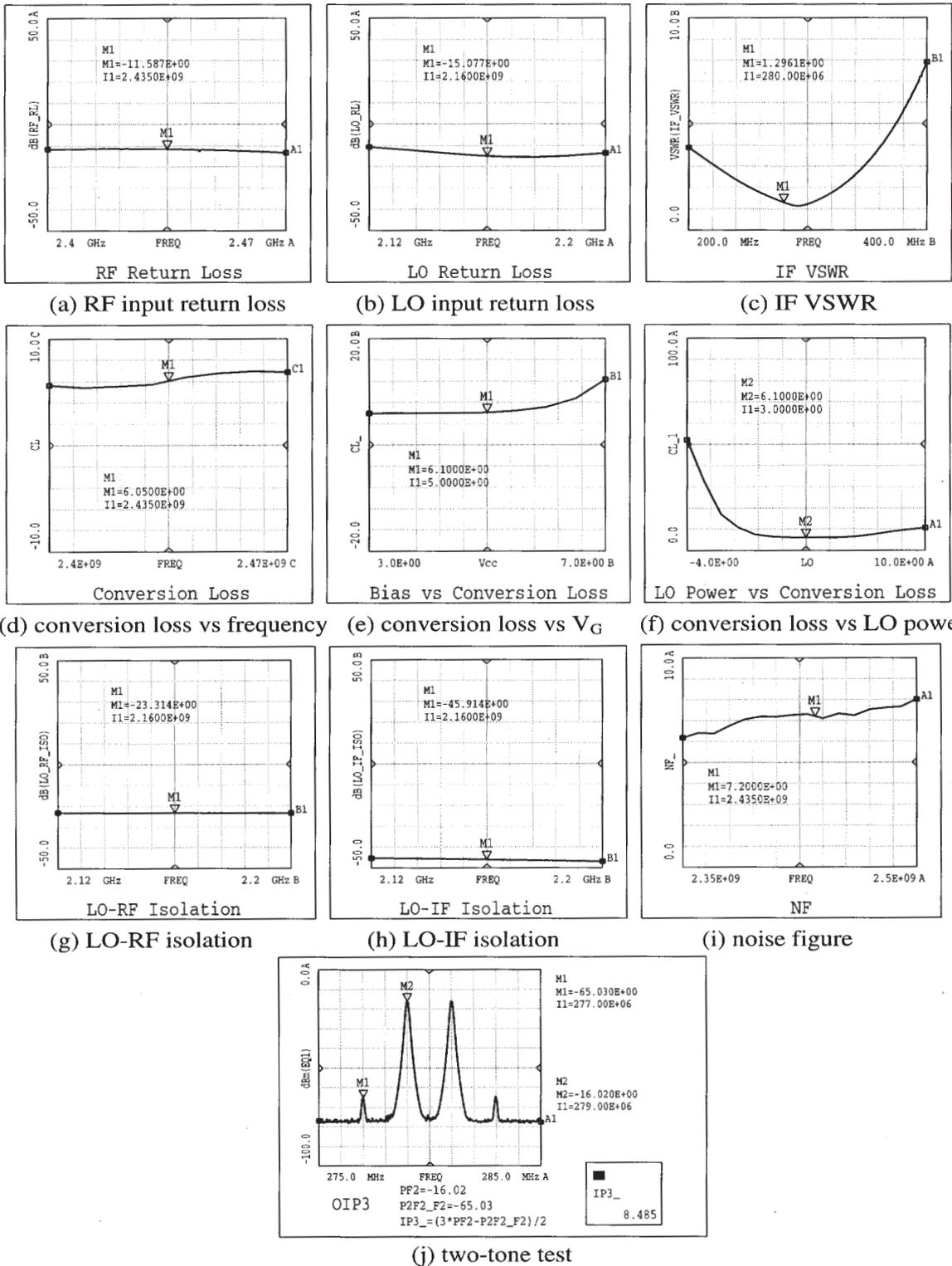
■ Figure 6. Measured characteristics of the 2.4 GHz single-ended resistive FET mixer.
