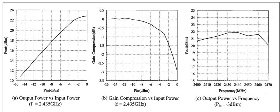
■ Figure 17. Measurement plots of transmit mode performance of the 2.4 GHz transceiver.
