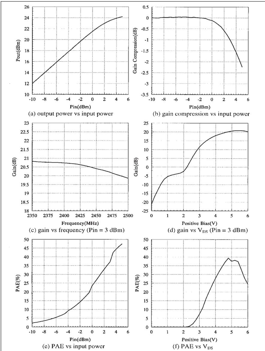
■ Figure 3. Measured performance of the 2.4 GHz power amplifier: (a) output power level, (b) gain compression vs. input power, (c) gain vs. frequency at 3 dBm input power, (d) gain vs. V<sub>DS</sub> at 3 dBm input power, (e) power-added efficiency (PAE) vs. input power, and (f) PAE vs. V<sub>DS</sub> at 2.435 GHz.
