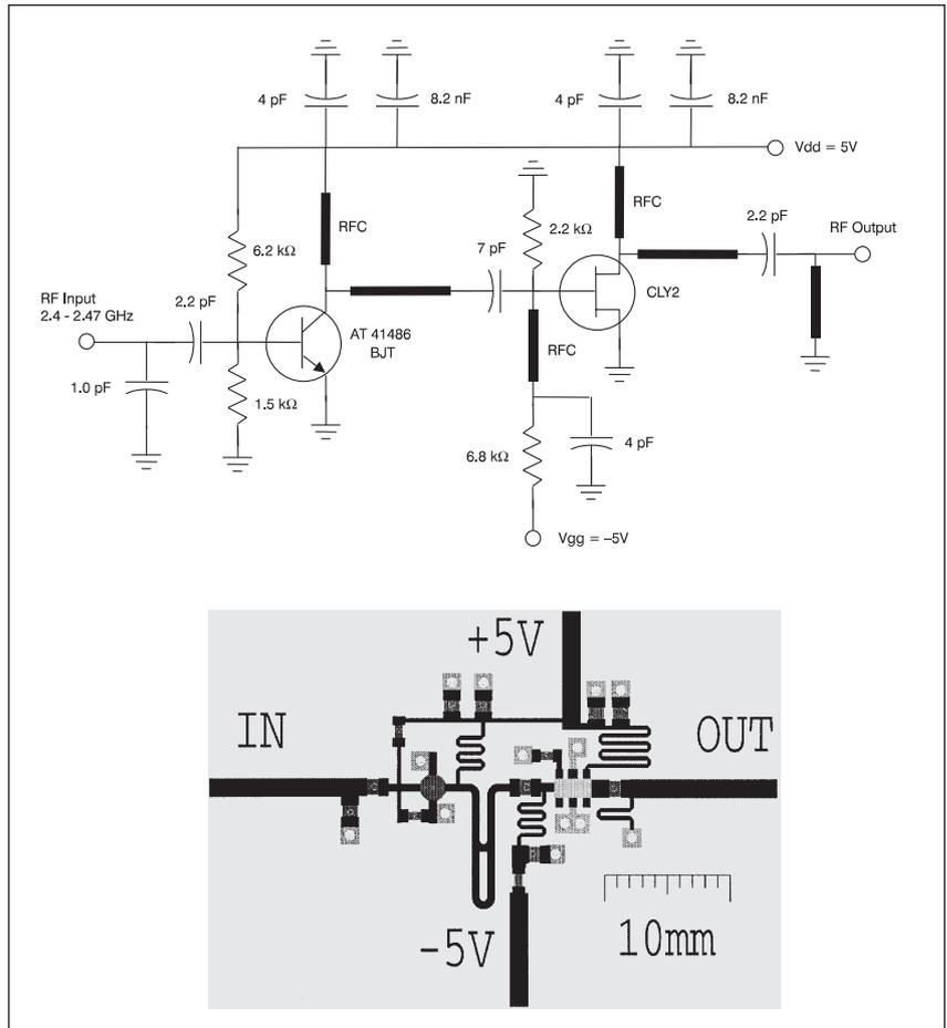
■ Figure 2. 2.4 GHz two-stage power amplifier — circuit diagram (top) and board layout (bottom).
