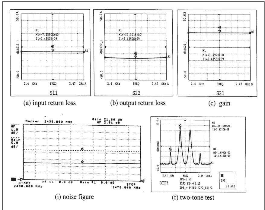
■ Figure 8. Measured characteristics of the 2.4 GHz two-stage low noise amplifier (LNA).
