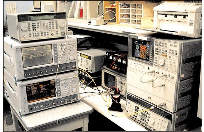
■ Figure 16(b). The test setup: Anritsu MG 3660A digital modulation generator and HP 89410A vector signal analyzer.
