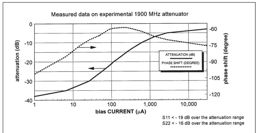
▲ **Figure 5. Attenuation range expected from the circuit of Figure 5. (Courtesy of Hewlett-Packard Company)**
