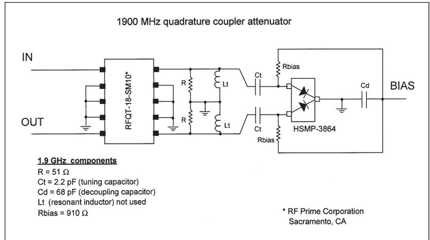
▲ **Figure 4. Circuit of a practical coupler-based attenuator. (Courtesy of Hewlett-Packard Company)**
