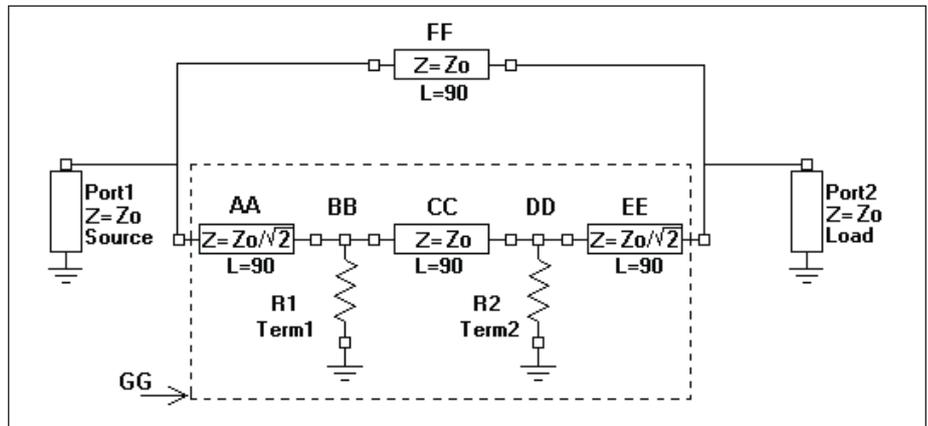
▲ Figure 2. Coupler schematic redrawn to emphasize two-port structure.
