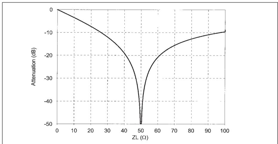
▲ Figure 3. Attenuation values for  $Z_L$  from 0 to  $2Z_0$ .
