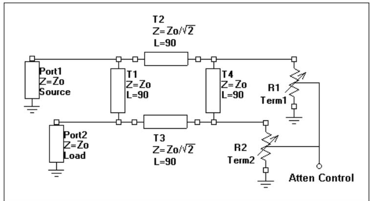
▲ Figure 1. Configuration of the coupler as an attenuator.
