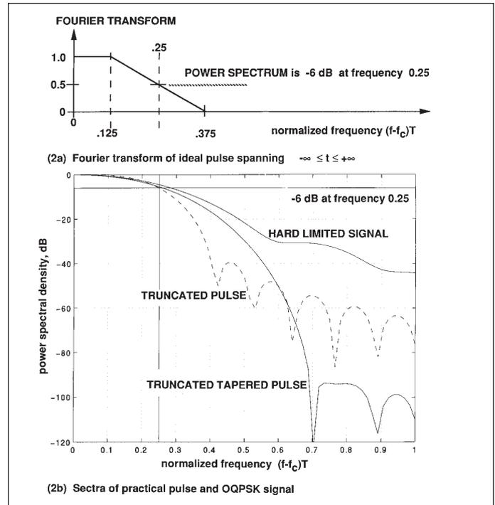
■ Figure 2. Spectra for data signals, all normalized to 0 dB at  $(f-f_c)T=0$ . The truncated tapered pulse spectrum in (2b) is the actual signal spectrum for very small amplifier input power level.
