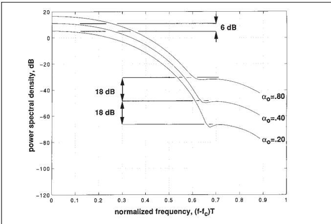
■ **Figure 3. Power amplifier output spectra for three drive levels 6 dB apart.**
