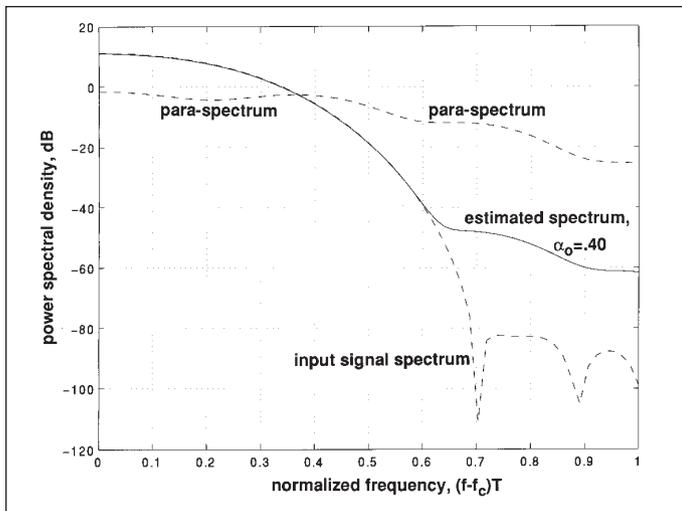
■ **Figure 5. Estimated power amplifier output spectrum for  $\alpha_0 = 0.40$ , based on the sum of input signal spectrum and para-spectrum.**
