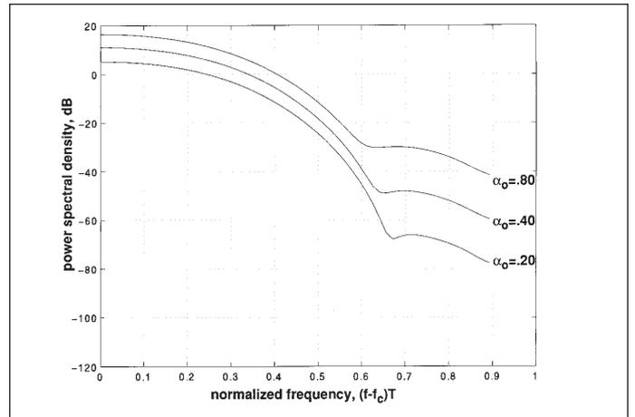
■ **Figure 4. Estimated power amplifier output spectra for three drive levels 6 dB apart, based on cubic approximation to amplifier nonlinearity.**
