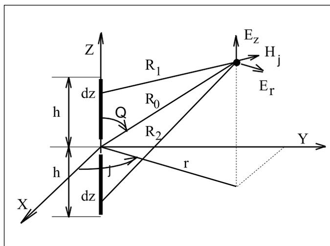
▲ **Figure 1.** A symmetric dipole in rectangular coordinate system.
