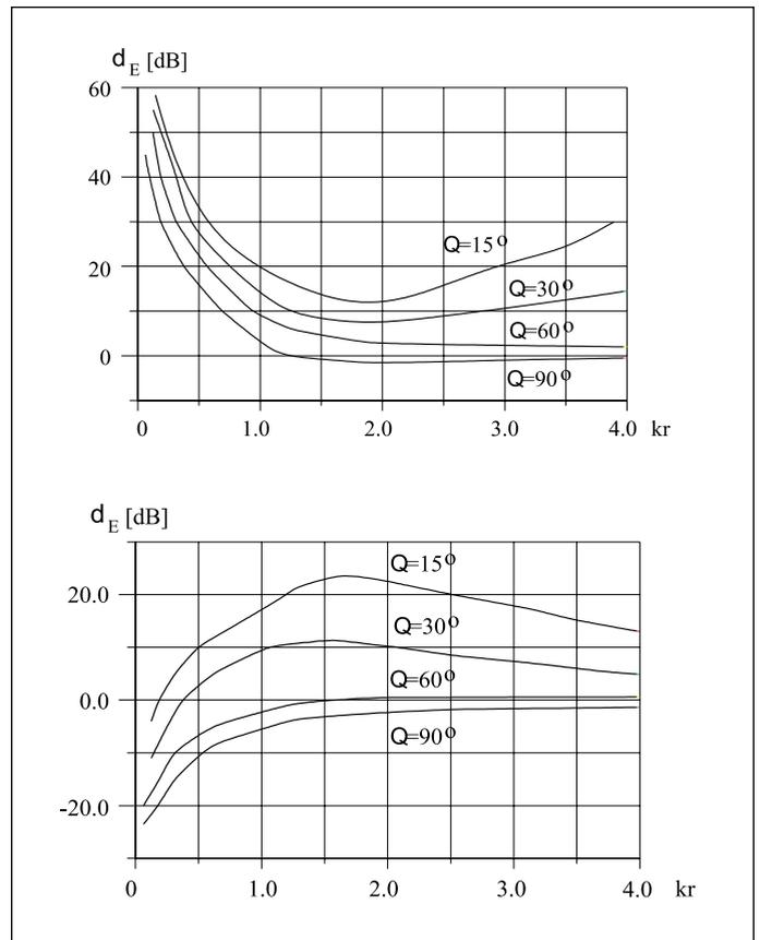
▲ **Figure 3.** Error  $\delta_E$  around a half-wave (top) and a full-wave dipole (bottom).
