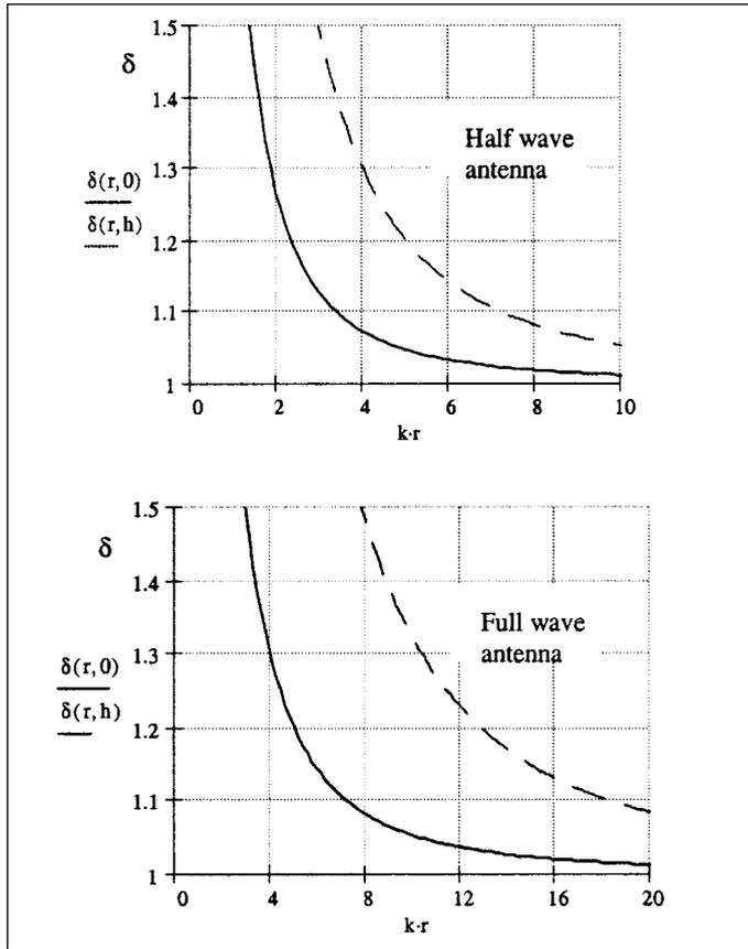
▲ **Figure 2** The factor  $\delta$  as a function of  $k \cdot r$  for the dipole center (continuous) and its end (dashed).
