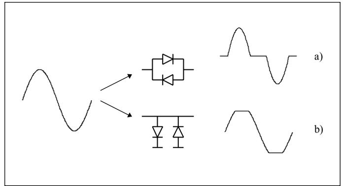
▲ **Figure 4. Two basic wave-shaping directions to create odd harmonics (the diodes are idealized as ideal switches with some forward voltage).**
