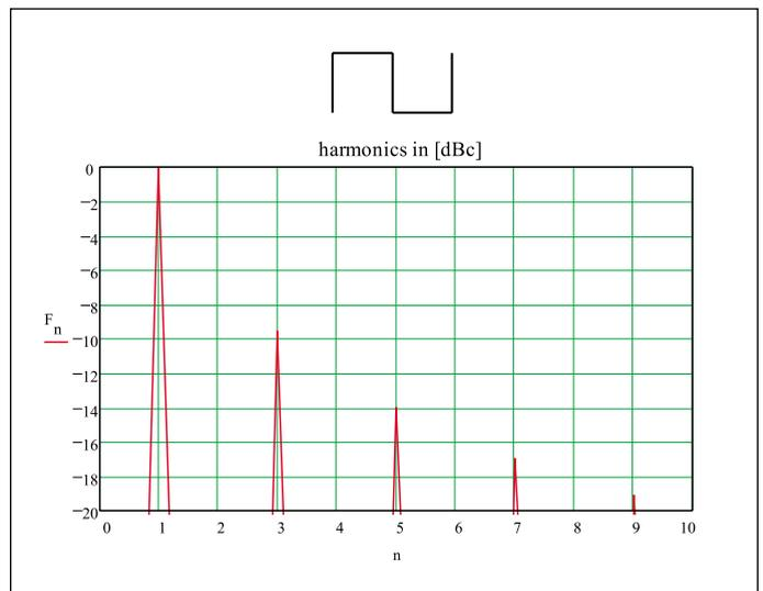
▲ Figure 6. The spectrum of rectangular wave: F3 level of -9.5 dBc, F5 of -14 dBc.
