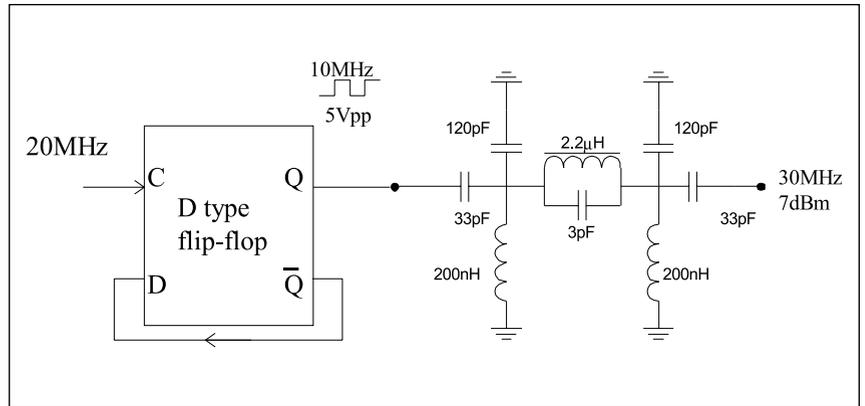
▲ **Figure 7. The frequency tripler 10 to 30 MHz example, with the ideal, input 10 MHz square-wave generated by a 74ACT74 implemented as a divide-by-two.**
