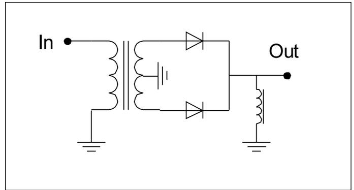
▲ Figure 2. Basic wide-band frequency doubling circuit.
