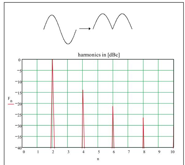
▲ Figure 1. Illustration of frequency doubling by wave-shaping with spectrum analysis results (DC component neglected).
