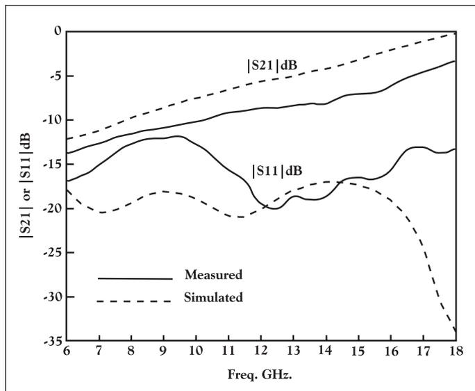
■ **Figure 4.** Insertion loss and return loss performance of the equalizer circuit.
