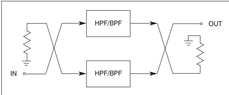
■ **Figure 2.** Lange couplers can be used with two filters to obtain good input and output match over an octave band.
