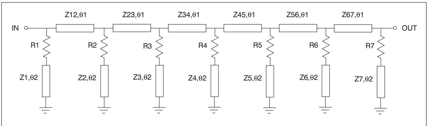
■ **Figure 3.** Cable Loss Equalizer topology using series stubs and resistively-loaded shunt stubs.  $Z_x$  is the line impedance and  $\theta_1, \theta_2$  are the electrical lengths.
