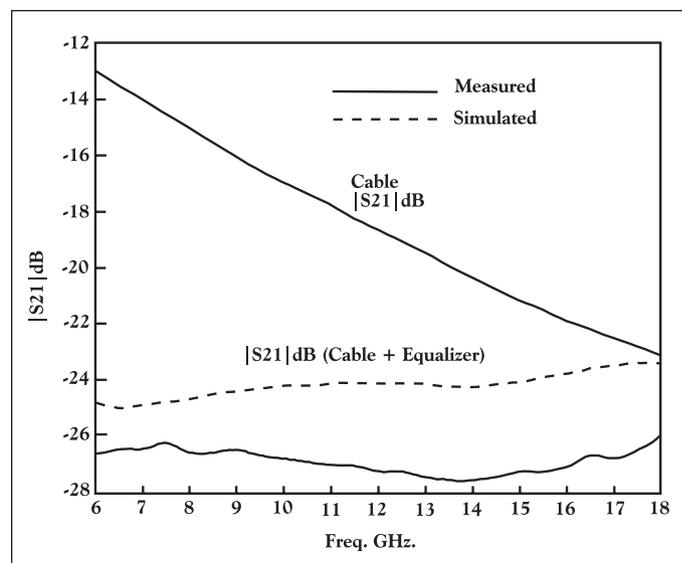
■ **Figure 5.** Cable attenuation and cable plus equalizer performance.
