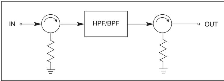
■ **Figure 1.** Isolators can be used to ensure a good input and output match.
