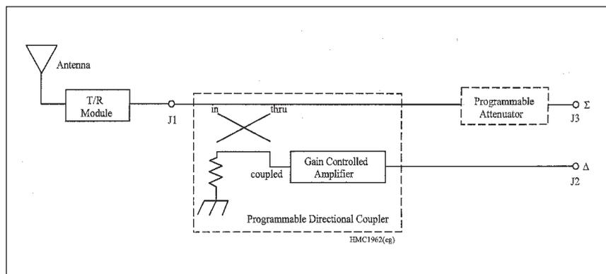
■ Figure 1. System block diagram, programmable coupler and attenuator.
