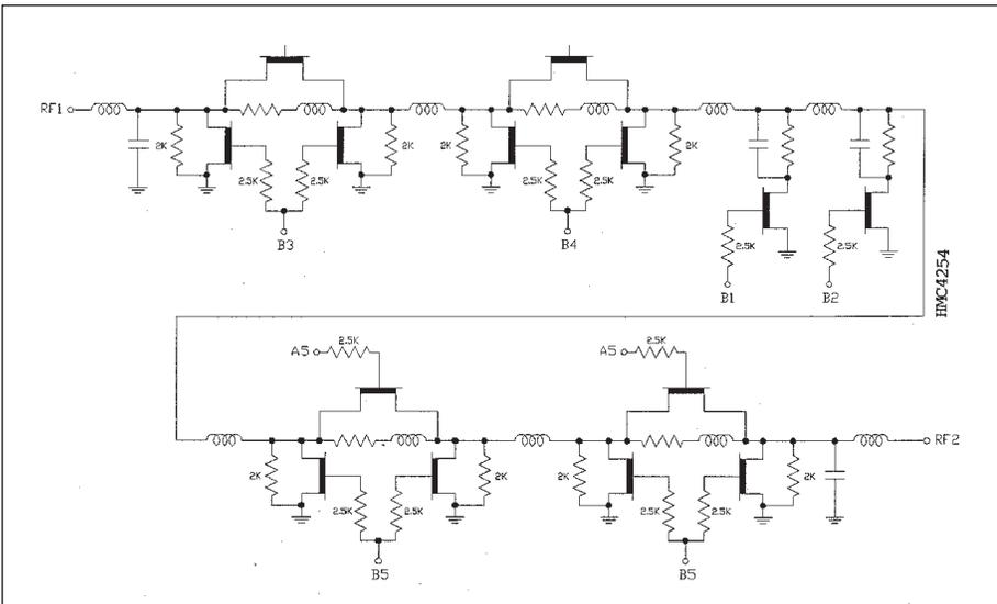
■ **Figure 7. Circuit diagram of the variable attenuator.**
