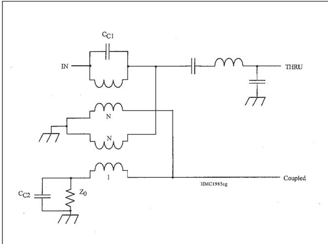
■ Figure 2. Circuit diagram, lumped-element MMIC coupler.
