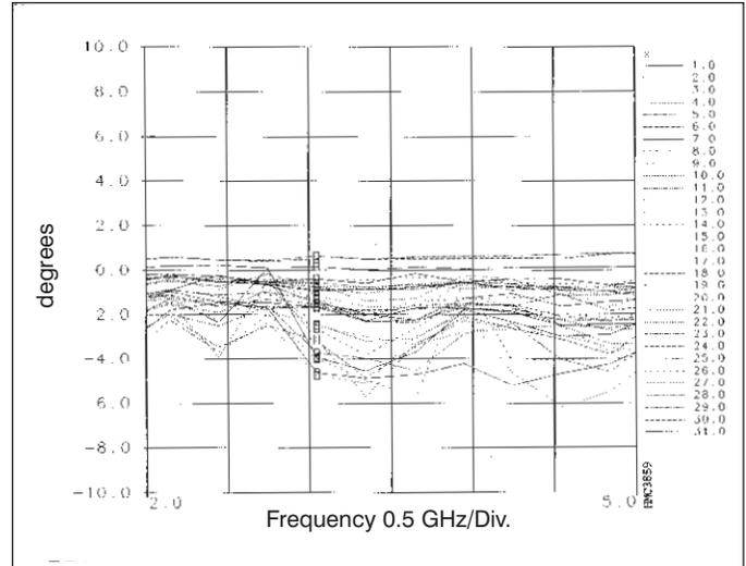
■ Figure 9b. Measured response of the variable attenuator MMIC: phase (deg.) normalized.
