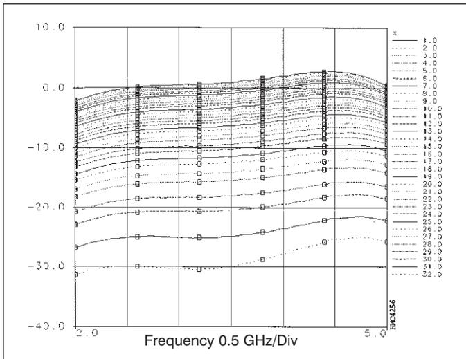
■ Figure 11a. Measured response of the programmable directional coupler: magnitude (dB).
