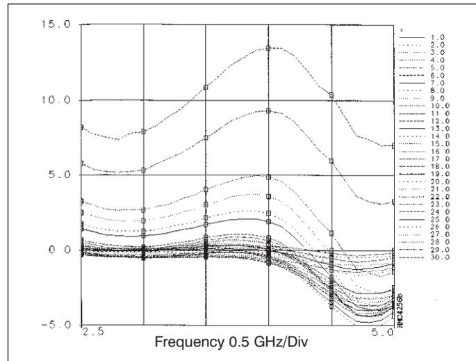
■ Figure 11b. Measured response of the programmable directional coupler: phase (deg.), normalized, two lowest gain states excluded.
