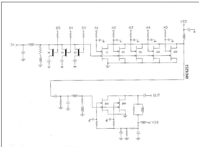
■ Figure 4. Circuit diagram of the variable-gain amplifier.
