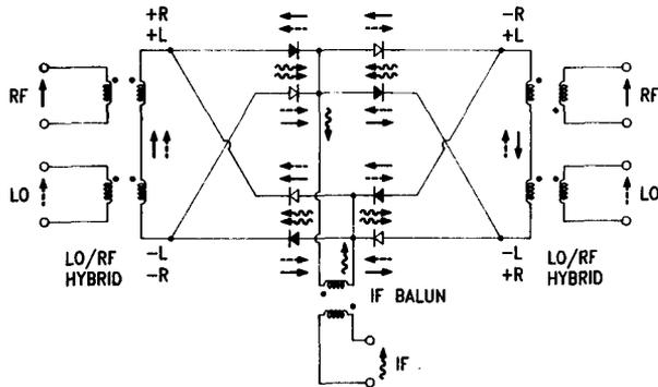
**Figure 2.** Equivalent circuit of a dual ring double-double balanced mixer.
