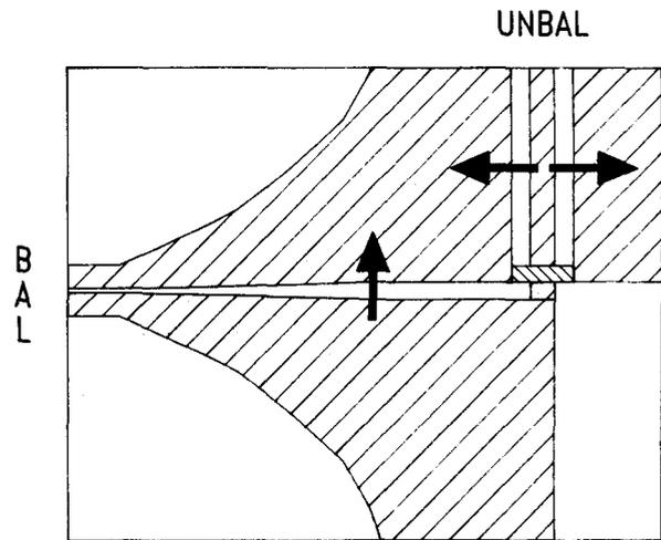
**Figure 8. The IF balun structure is formed by transitions from CPW to slot line to CPS.**
