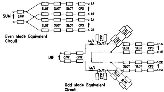
Figure 4. Odd and even mode equivalent circuits of the 180 degree hybrid.
