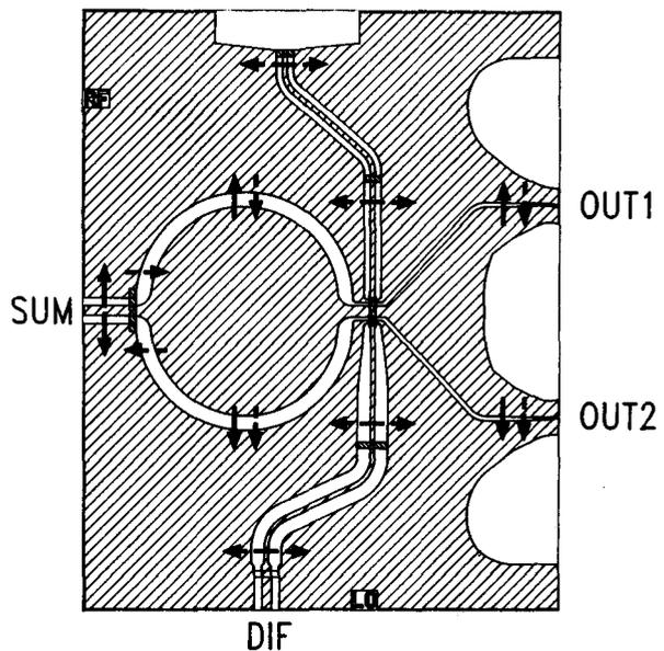
Figure 5. Layout of the 180 degree hybrid composed of CPW, CPS and slot lines.
