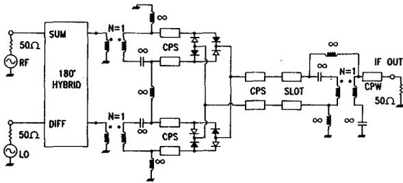
**Figure 9. Equivalent circuit used for harmonic balance analysis showing diode connections and infinite value L's and C's added to setup proper dc initial conditions.**
