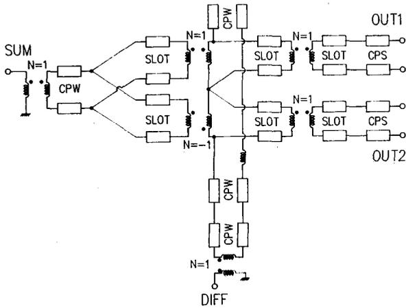
**Figure 6. Equivalent circuit model of 180 degree hybrid is obtained by super-position of the individual odd and even mode equivalent circuits of the device.**
