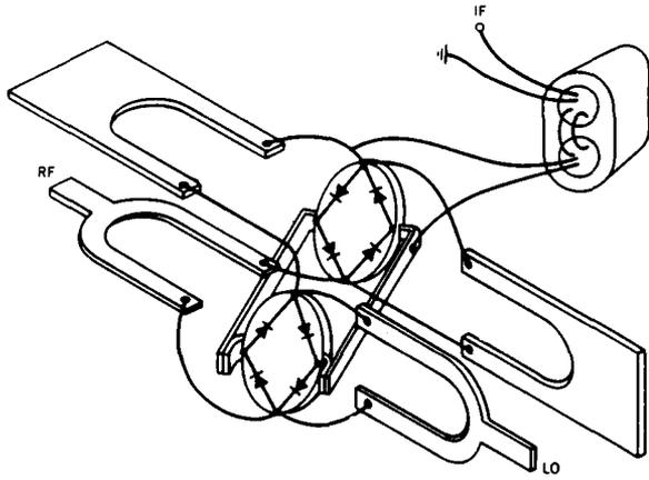
**Figure 1.** Example of a typical non-planar DDBM realization. Structures such as these are very difficult to realize in a MMIC format.
