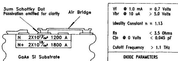
**Figure 10. Cross-section of Litton MMIC Mixer Diode showing the air bridge connection to the 3 micron Schottky dot.**
