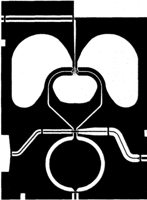
Figure 3a. Photograph of double-double balanced mixer chip showing RF, LO 180 degree hybrid, IF balun and dual diode ring. Chip size is 180x240x16 mils.
