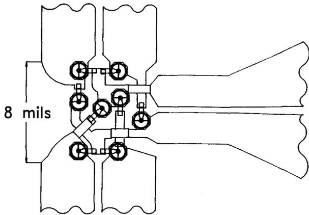
Figure 3b. Detail of dual diode ring showing connections to the RF-LO Hybrid and IF Balun.
