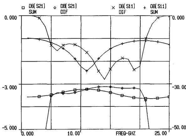
**Figure 7. Computed performance of 180 degree hybrid.**
