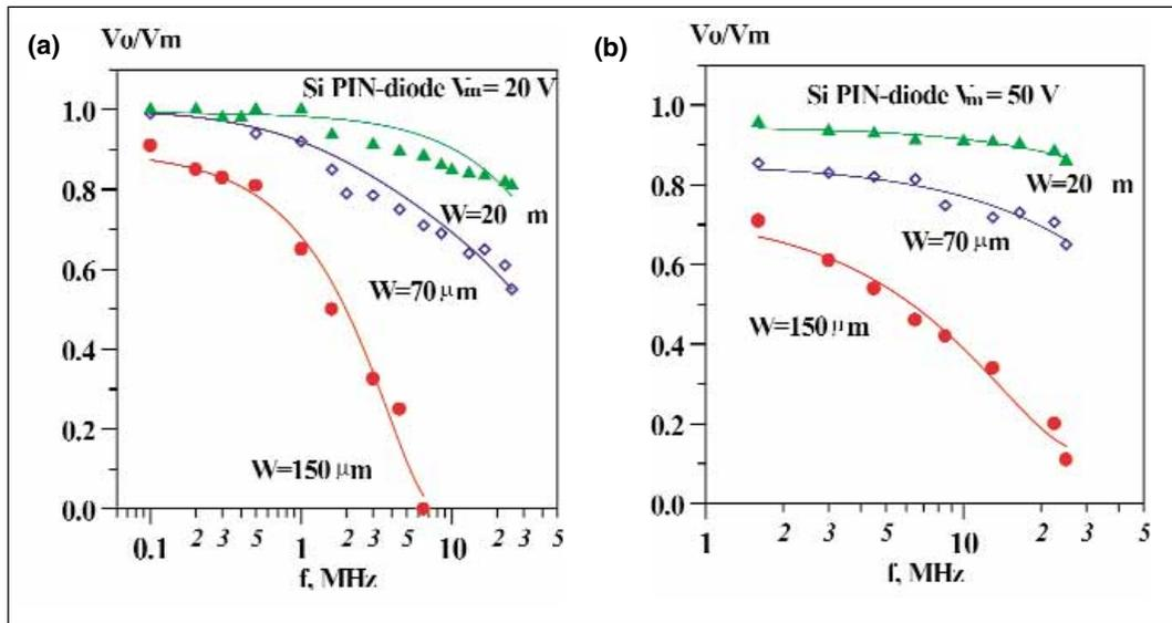
▲ **Figure 2.** Required DC reverse bias voltage versus frequency for PIN diodes with different i-layer thickness. (a)  $V_m = 20$  V; (b)  $V_m = 50$  V.
