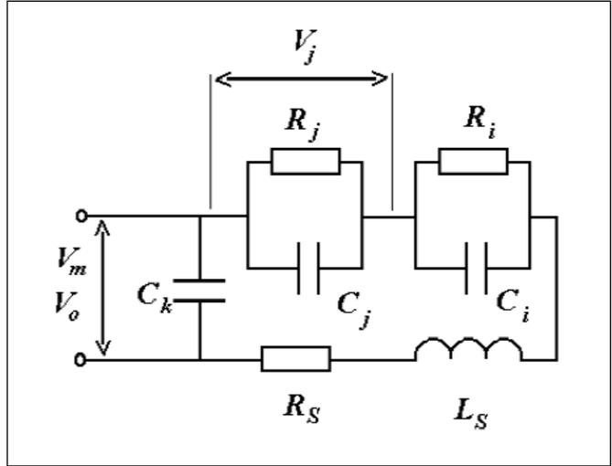
▲ Figure A2. Equivalent circuit of a PIN diode.
