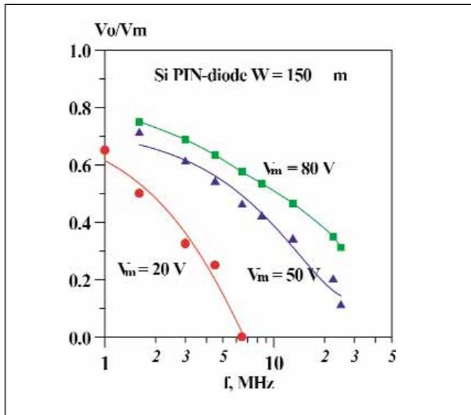
▲ **Figure 3.** Required DC reverse-bias voltage versus frequency of a 150  $\mu\text{m}$  PIN diode with a different input RF voltage amplitude.
