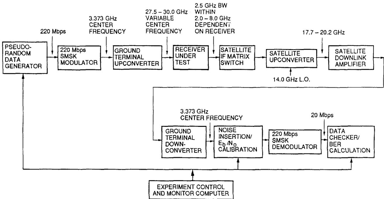
Figure 7. Diagram of the receiver bit error rate (BER) measurement system.
