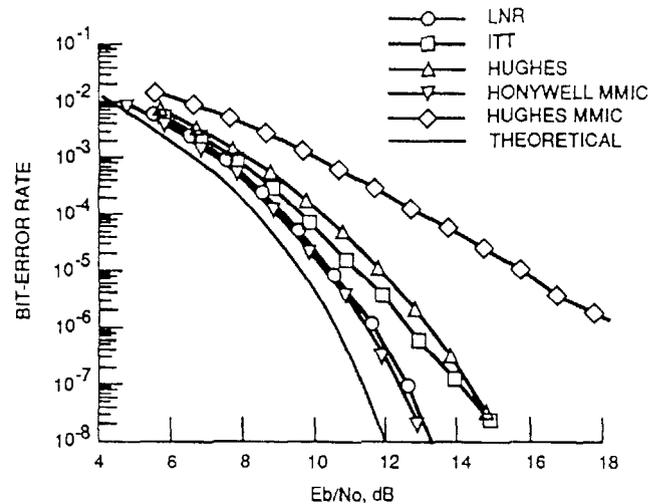
Figure 8. Measured BER for the five receivers when their input power is -30 dBm and the satellite high power amplifier is in saturation.
