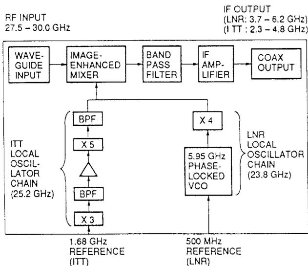
Figure 2. Diagram of the LNR Com. Inc and the ITT Defense Com. 30 GHz low noise receivers.
