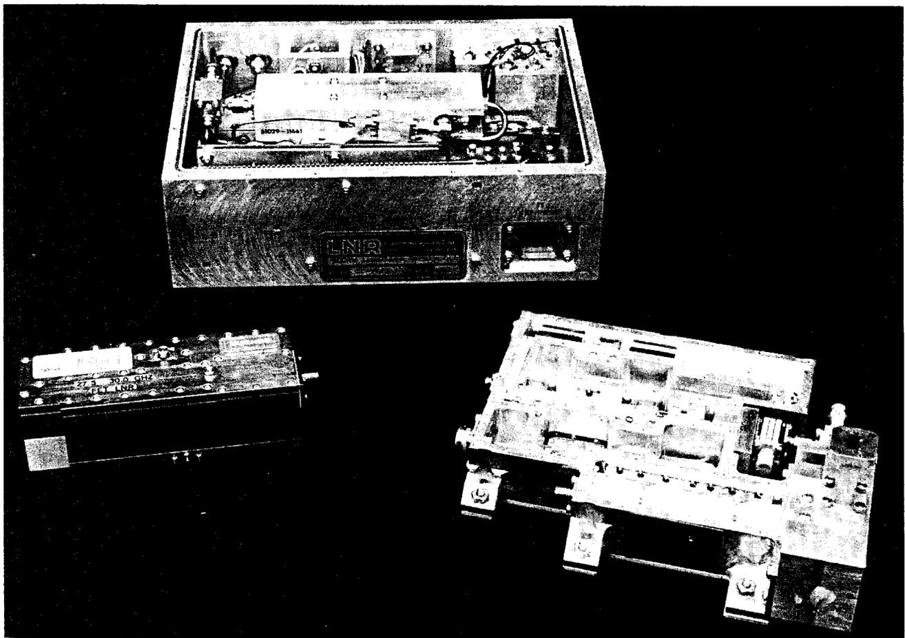
Figure 1. Photograph of the hybrid microwave integrated circuit (MIC) receivers built by (left to right) Hughes, LNR Com. Inc, and ITT Defense Com.
