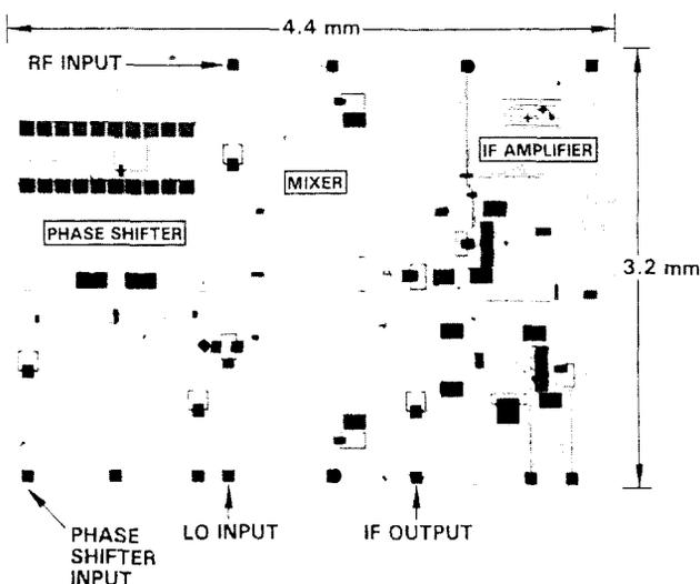
Figure 6. The Hughes monolithic receiver chip.
