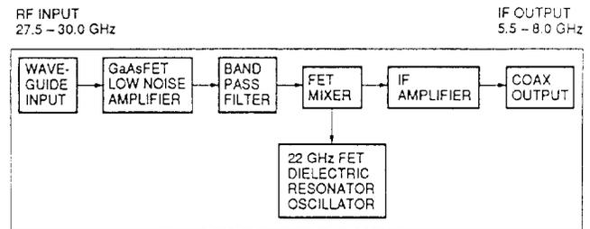
Figure 3. Block diagram of the Hughes MIC low noise receiver.
