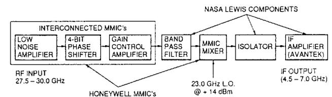
Figure 4. The Honeywell MMIC receiver test configuration.
