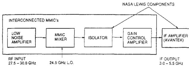
Figure 5. The Hughes MMIC receiver test configuration.
