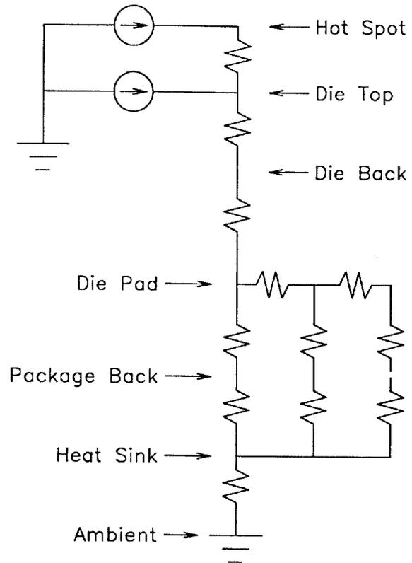
Figure 5. Thermal network used by TempEst
