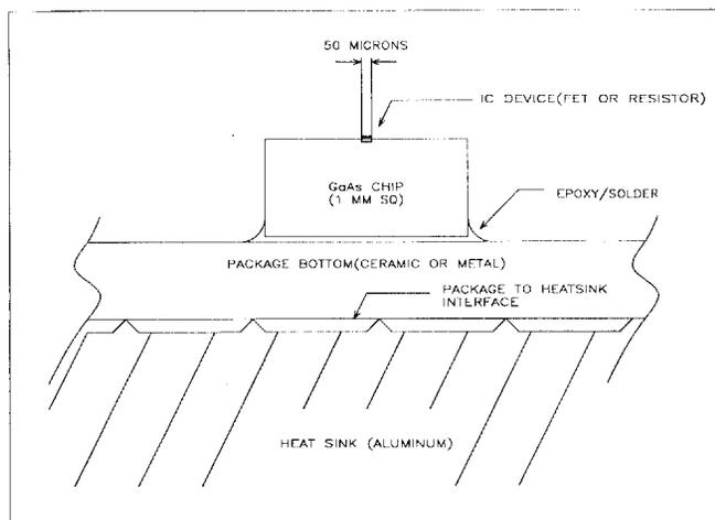
**Figure 1. To-scale generic thermal environment for a typical GaAs IC chip.**
