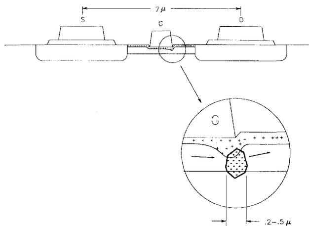
**Figure 2. Approximate location of the heat generating region of an FET.**
