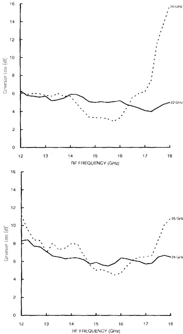
**Figure 8. Mixer conversion performance for a fixed 20, 22, 24, and 26 GHz LO frequency at about +14 dBm.**
