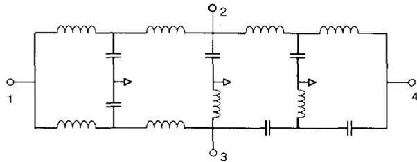
Figure 4. The 180 degree was implemented using fourth order high/low pass filter structures.
