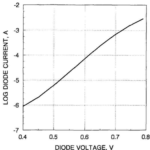
**Figure 6. Measured current-voltage characteristics of the Schottky diode.**
