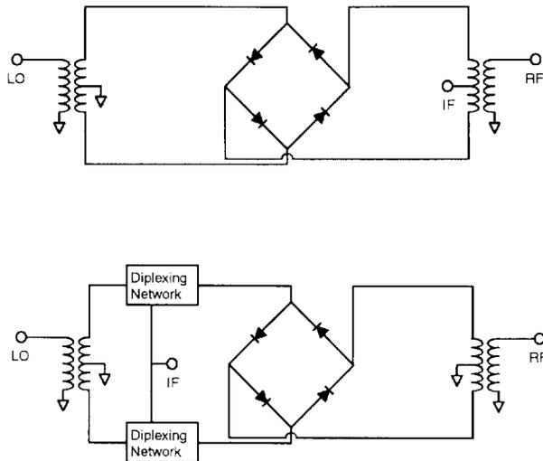
**Figure 1.** Most MMIC diode mixers are based on four diodes arranged in a star configuration which are connected to two baluns. The IF signal can be extracted by either of two means, a) the fourth port of the baluns, and b) by diplexing the IF from either the LO or RF signal.
