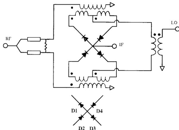
**Figure 2.** The new mixer is based on a topology where the four diodes are arranged in a star configuration.
