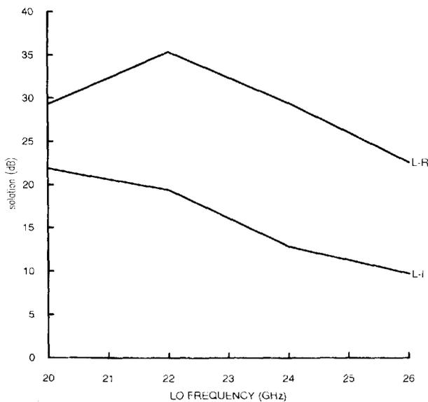
**Figure 9. Measured mixer isolation between LO and RF ports and between LO and IF ports.**
