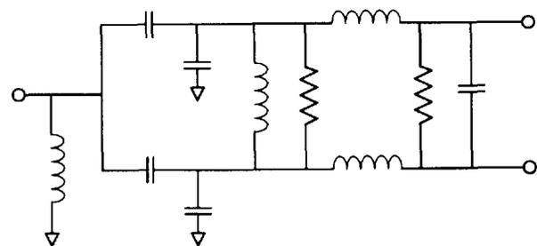
**Figure 3. The power divider was realized using a lumped element topology based on a minimum element bandpass structure.**
