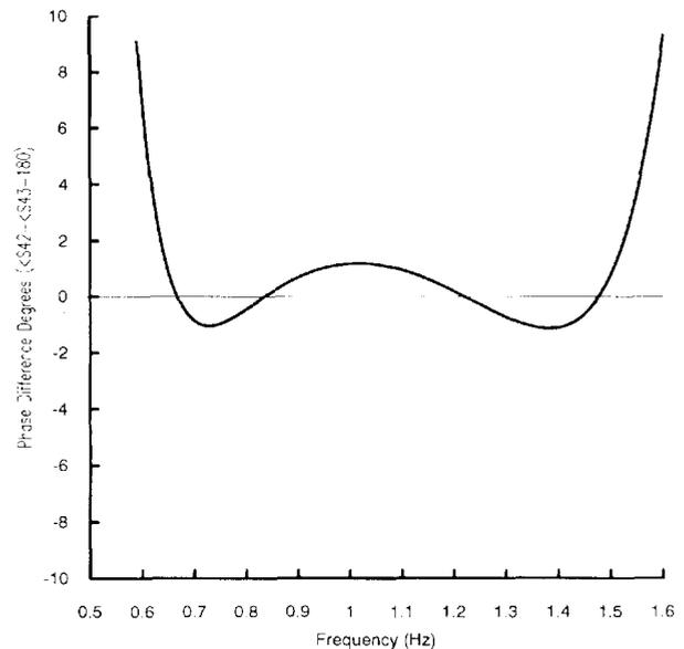
Figure 5. Response of low pass prototype 180 degree hybrid with a center frequency of 1 Hz and 1 ohm impedance. a) Insertion response of S21, S31, S42, S43. b) 180 degree phase response.
