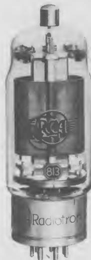
High-Power Sensitivity and a power output in Class C service of 260 watts make the RCA-813 an excellent tube for medium power rigs. Elimination of neutralization in adequately shielded circuits and a driving power of less than 1 watt are other important features.
