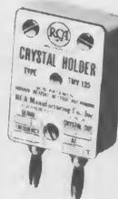
Unusually high-power output, plus an extremely low temperature coefficient, make the RCA V-Cut Crystals ideal for amateur use. Crystals are supplied within 0.1% of specified frequency and are calibrated to an accuracy of 0.005% at calibration temperature. Temperature coefficient is 4 cycles
