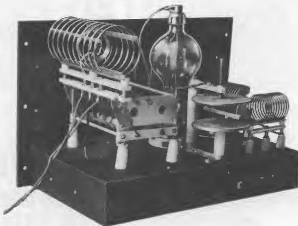
W2HNP of Roselle Park, New Jersey, rates a five for this fine photo. Tube line-up consists of an RCA-6L6 crystal oscillator, RCA-809 buffer amplifier, and on RCA-806 final with the famous Enclosed Tontolum Anode. Says W2HNP, "the 806 is working swell on all bands—operates on both phone and c.w. with between 400 to 600 watts input." More power to you, Om—if you need it!!
