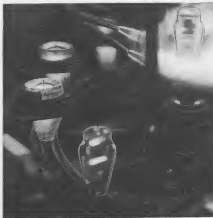
RCA-811's and 812's are sealed and pumped free of air in a spectacular run through the famous SEALEX machine. More adept than human hands, more accurate in vacuum control than the element of human judgment, this machine produces finished tubes that are uniform both in characteristics and in quality.
