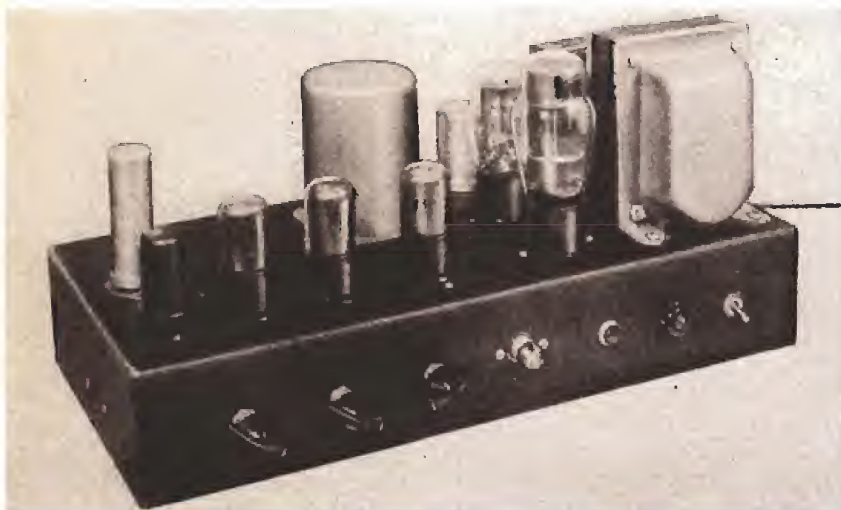
Featuring a low cost resistance-coupled driver stage and independent tone-control circuits for bass and treble, the amplifier delivers 10 watts of audio power with less than 2% distortion
