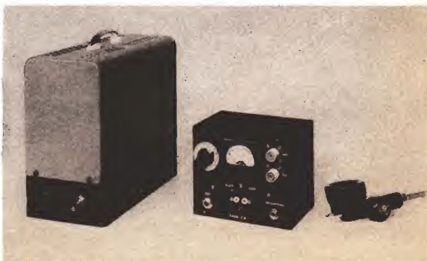
This efficient looking rig features the new crystal reactance system for obtaining frequency modulation. It's a natural for Amateurs who do a lot of travelling by automobile.
