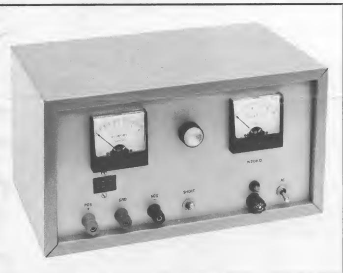
Exterior view of W2OK0's power supply shows lineup (left to right, bottom) of positive, ground, and negative terminals; shorting switch; fuse and pilot light (above fuse); and line-voltage switch. Unmarked control knob between the two meters is used for setting desired voltage.
