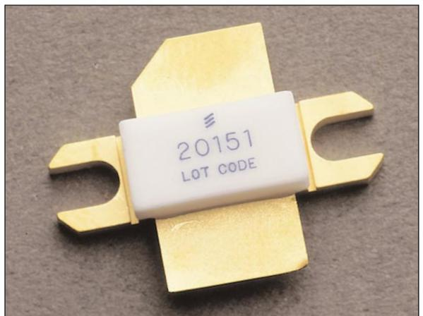
■ **Figure 1. A silicon bipolar RF Power transistor capable of delivering 45 W of output power at 1.8 to 2 GHz for PCN/PCS systems.**
