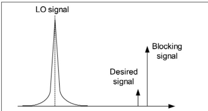
▲ Figure B(1). RX input signals and LO with phase noise spectrum.
