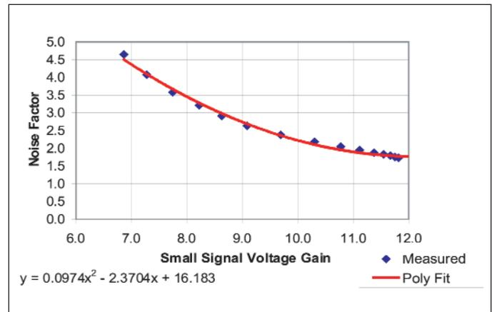
▲ Figure 7. Noise factor versus small signal gain.
