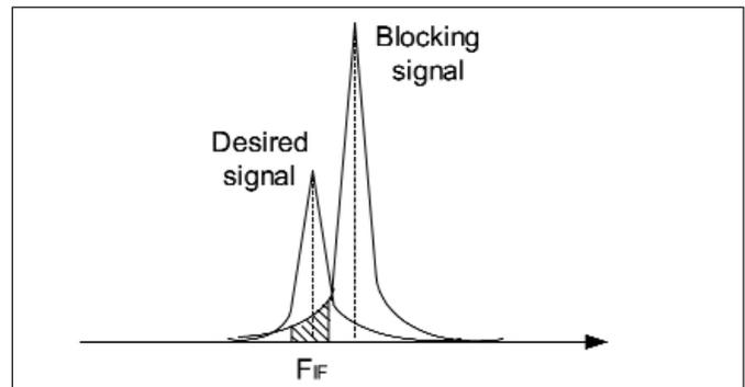
▲ Figure B(2). Signals downconverted to IF, with overlap of reciprocally mixed noise.
