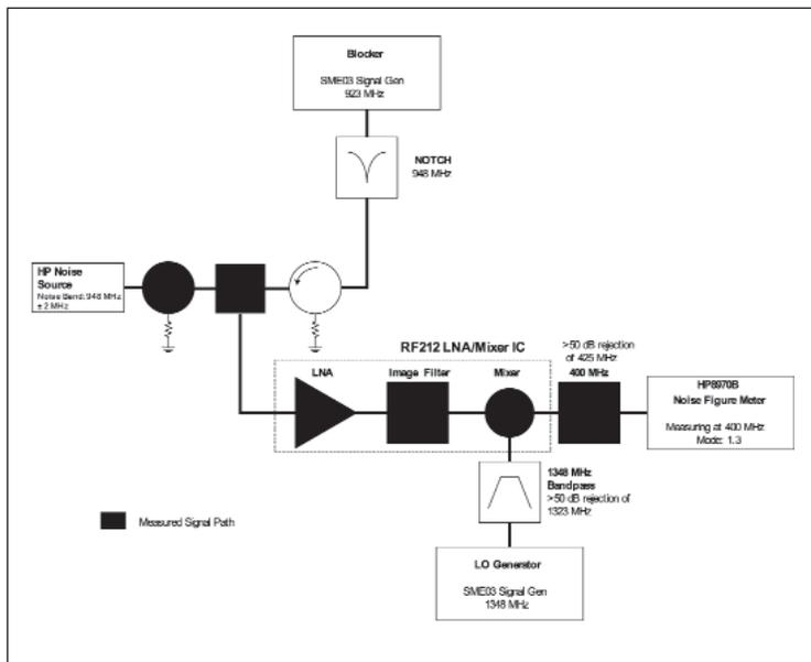
▲ Figure 5. Test setup to measure blocker effects.
