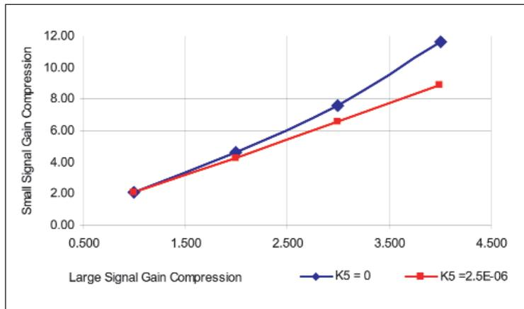
▲ **Figure 2. Small signal gain compression, with  $k_3 = .0025$ .**
