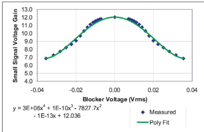
▲ Figure 6. Small-signal gain versus blocker voltage.
