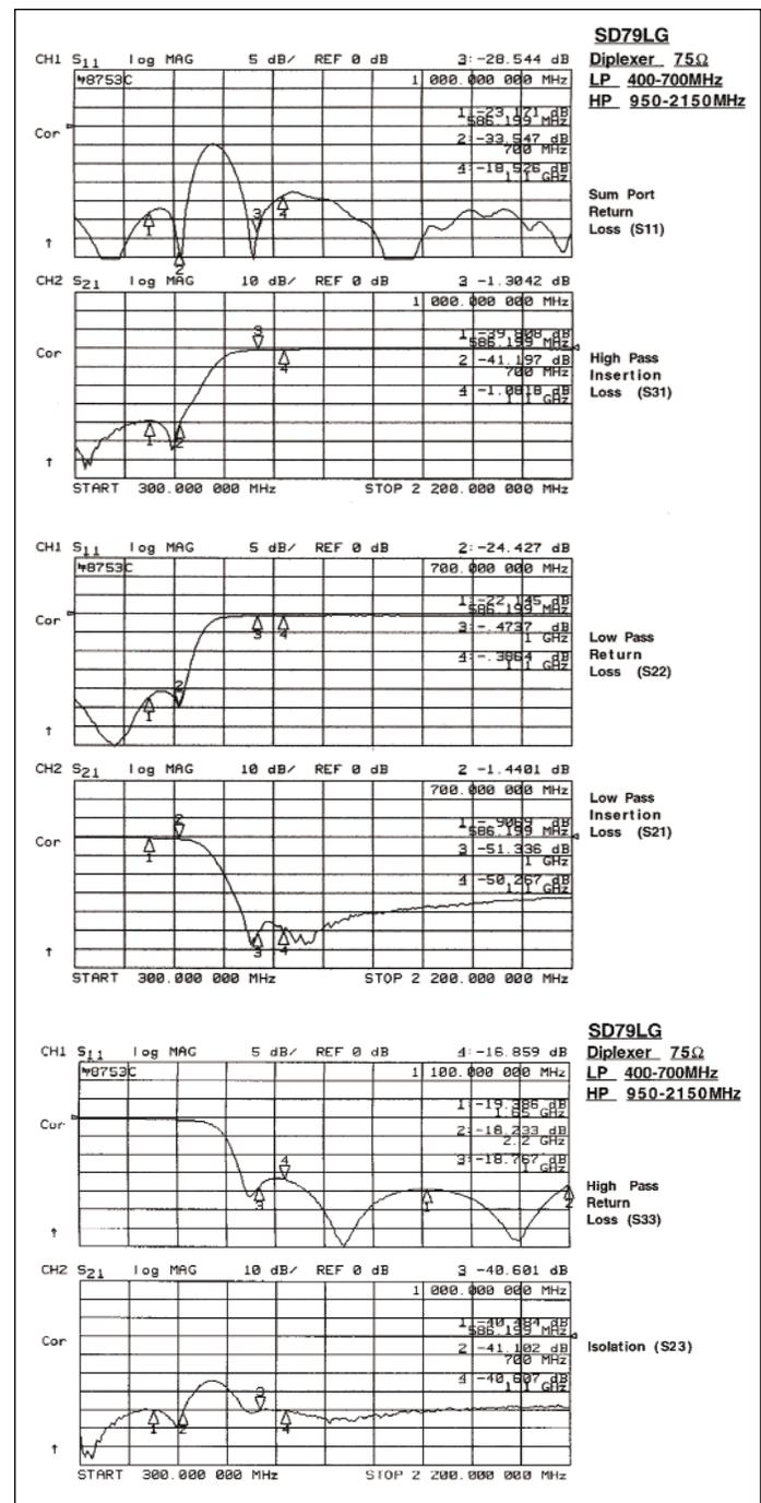
▲ Figure 5. Actual network analyzer plots of the SD79LG.
