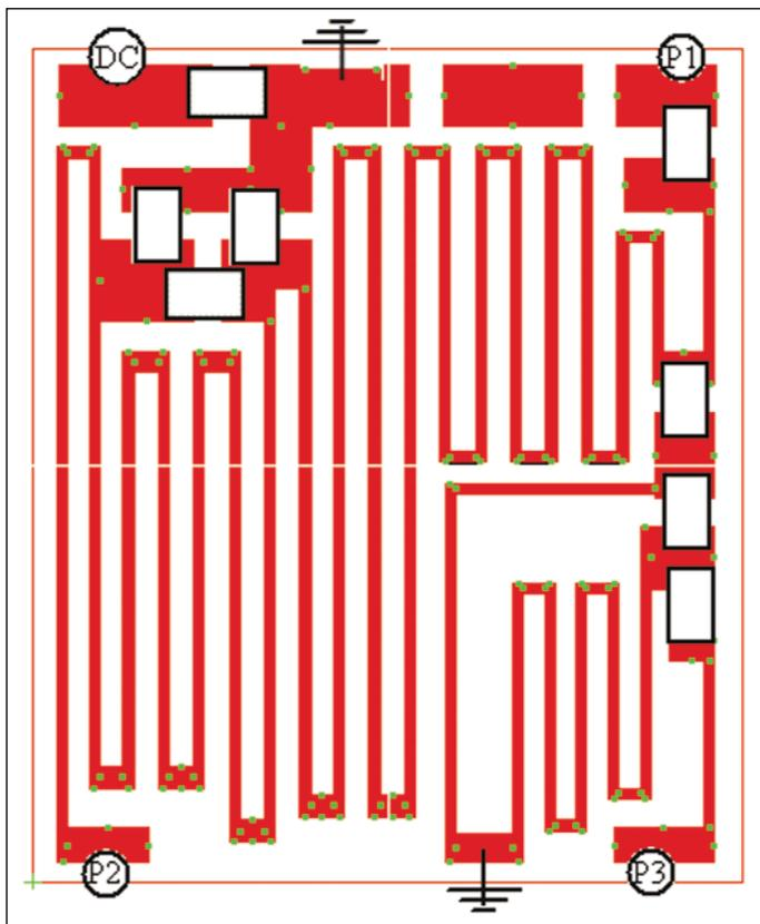
▲ Figure 4. Finished trace layout with capacitors.
